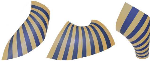
Figure 20: Isometric bending of a geodesic model. One of the geodesic models contained in Fig. 17 undergoes experimental isometric deformations after it has been built from paper. Bending strip models has many more degrees of freedom than isometric bending of meshes (false color photos of paper models).
