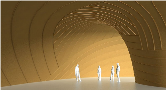
Figure 17: Geodesic D-strip models (in total five) which cover the interior of a freeform surface.
